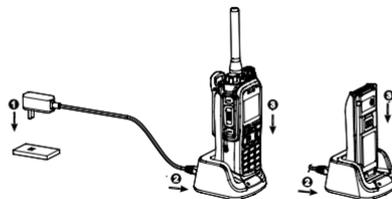
During charging, the LED indicator on the charger will indicate the charging status. The charging begins when the charger LED glows red. When charging is complete, the charger LED glows green.
