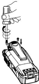
To remove the belt clip, loosen the screws. Please keep the screws properly. It is recommended to replace them to the terminal.
